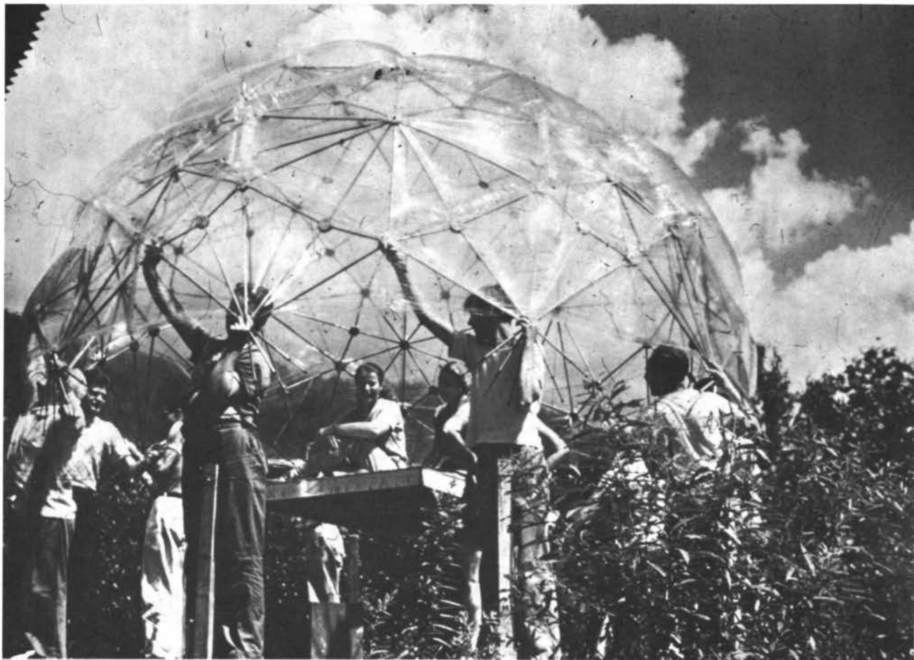
(P-1-9) Here we have a platform suspended from a geodesic dome. Three people are sitting on the platform. Students are testing the way earthquakes would affect such a structure by alternately removing the separate students' supports along the base of the dome. We found that the stresses induced by this wave generating pattern were absorbed in the first row of triangles above the equator.
